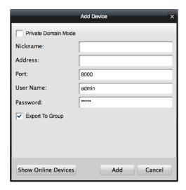
If you check the Private Domain Mode checkbox, you should enter the DNS address and Device Domain Name as well.
