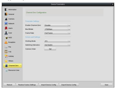
On this page, you can enable/disable channel-zero coding, set the encoding parameters(max bitrate and frame rate), screening-split settings (working mode and switching intervals) and camera order for displaying.
