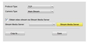
To configure the steam media server, check Obtain Video Stream via Stream Media Server checkbox .
