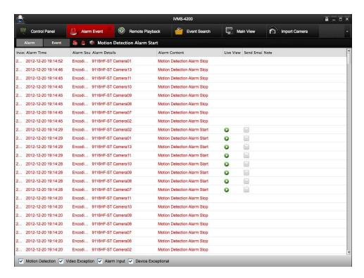
As shown in the figure above, in the alarm log display panel, there are 4 different alarm types: "Motion", "Video Abnormal", "Alarm Input" and "Device Abnormal".
