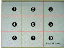
Use the mouse to click on the video image, and then drag the mouse to different directions by following the arrows displayed on the video: • Upper Left; • Up; • Upper Right; • Left; • Right; • Lower Right; • Down; • Lower Right. The PTZ will move to the direction as the arrow goes.
