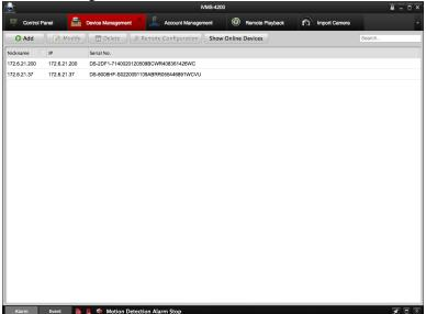
3. Create a nickname for the device and then input it with other information, the User Name and Password are admin and 12345 respectively and the port number is 8000 by default.
