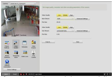
On this page, you can configure parameters for main stream and sub-stream separately. You can set video quality and resolution on the main interface. To configure steam type, bitrate type, max bitrate, frame rate, frame type, frame interval and encoding type, please click Advanced Settings button to enter advanced setting interface.
