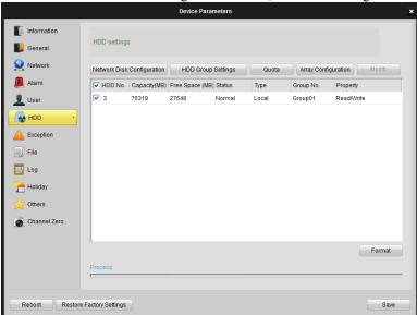
3. Click format the HDD installed in the device. And the process bar shows the formatting process of the HDD.
