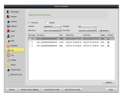
Captured pictures and record files stored on local devices can also be searched, played back and backed up. Picture types include motion detection, alarm, continuous capture and etc.
