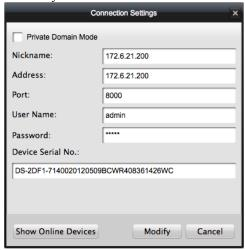
Click configuration icon to delete the selected device and you can also configure the settings of the device by clicking Remote Configuration. For the detailed procedures of remote configuration, please refer to 4.3 Remote Device Management and Configuration.
