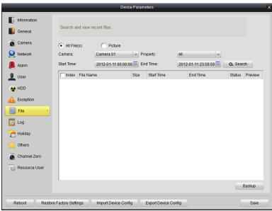
If the device supports remote backup function, you can also select files and click Backup to back up all the selected record files.
