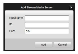
3. Create a nick Name, enter IP address of the PC on which the stream media server is running, and Port number (the Port 554 is the default RTSP port number), and then click **Add** to save it.
