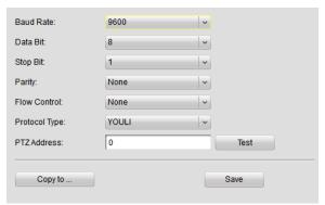
*Note:* The PTZ parameters should be consistent with the settings of the PTZ on the DVR or IP camera side to ensure valid PTZ control.
