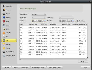
If the device supports remote backup function, you can also select logs and click Backup to back up all the selected log files
