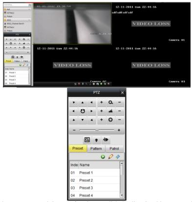
Click on those directional buttons to control the PTZ function, or click the directional buttons on the PTZ control panel. You can also control the PTZ direction by the directional buttons on your keyboard.
